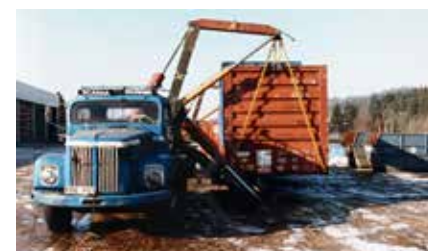
A new SL 30 test lifts 40 tonnes (88100 lbs) on Hammar's tractor unit in the mid-80s. At this time, new sideloaders were painted after they had been mounted and tested.
