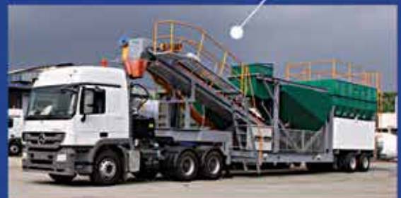
Buffalo Mobile Batching Plant Uses JOST Landing Gear & TTK Trailer Component
