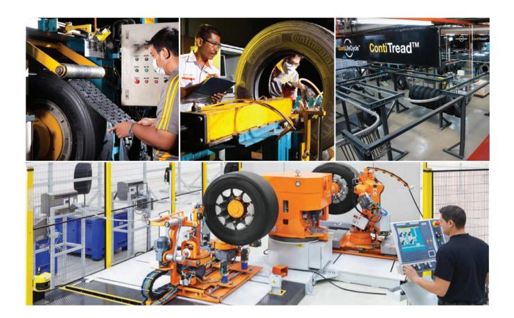
Before a tyre is retreaded, stringent inspection will be carried out to ensure the casing is fit for a safe second life. For the all-important initial inspection, several methods are used. These include visual inspection, nail-hole detection, and Shearography, also known as X-Ray in some markets. Only if these tests are conducted according to the highest quality requirements, can the casing be released for retreading.
