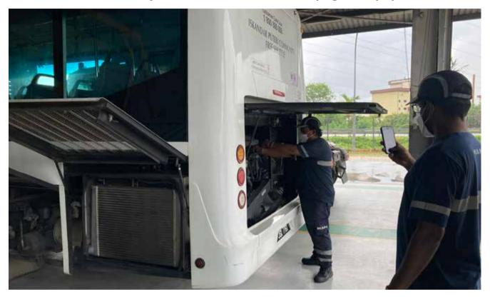
number of issues arise when vehicles are parked for extended periods of time. The flat battery is an obvious problem, one that is quickly fixed, but it is not the only issue that needs to be considered when re-starting your fleet. Rodents may have gnawed on pipes and wires, filters may need replacing and oil changing. We spoke to Navin Manogaran, Head Customer Service Management, General Manager, MAN Truck & Bus (M) Sdn Bhd (MTBM) about their current campaign to help the industry to "Rise Back".
