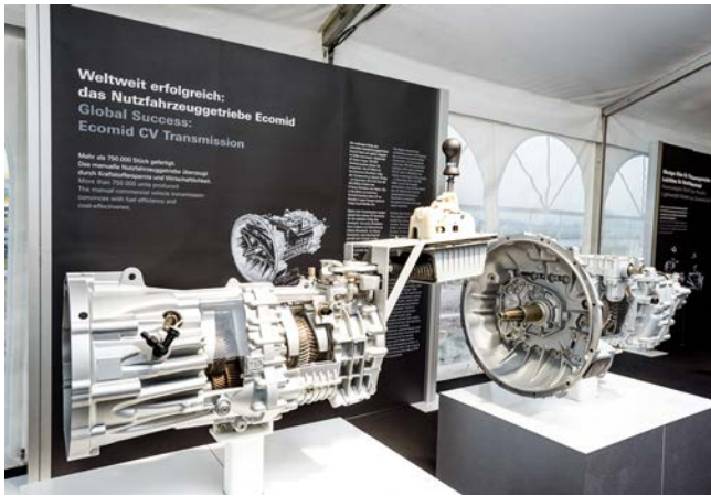
ZF Ecomid manual transmissions for commercial vehicles on display at the ZF Trade Press Conference 2014
