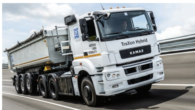
The TraXon hybrid transmission from ZF reduces fuel consumption by up to 15 percent in truck prototypes from Kamaz
