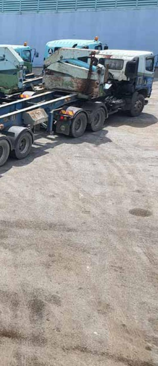
The team at Intercargo saw the unique benefits that adding sidelifters to the fleet would bring to the business. The units are able to load and unload a container on the ground instead of on the back of a trailer.
