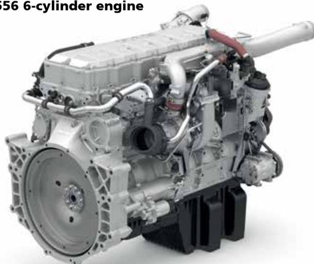
Meeting the Euro 6d emission standard was another development goal. MAN opted for a compact and robust design without exhaust gas recirculation. The SCR system enables the brand to implement higher NOx figures than the D20.
