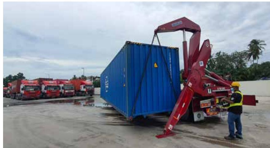
Another drawcard for Artha was the versatility that the Steelbro units provide including trailer transfer and double stacking. All Steelbro Sidelifters can double stack both 20' and 40' containers. According to Viswanathan this has been a problem solver "Our space constraint issue was solved with Steelbro double stacking."
