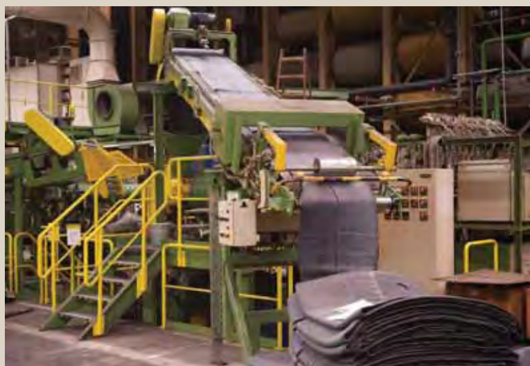
The various components of the tyre are being created from rubber mixtures, using extrusion
