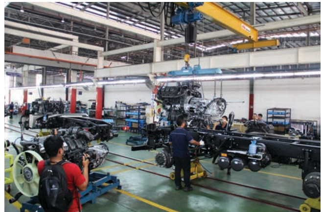
A marriage made in Pekan - Frame and engine come together
