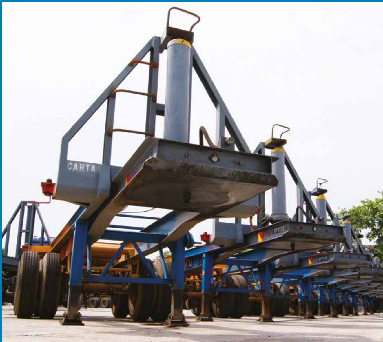
Front end piping cyclinder
