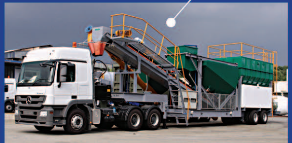
Buffulo Mobile Batching Plant Uses JOST Landing Gear & TKK Trailer Component
