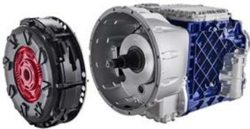
*The I-Shift Dual Clutch as seen from offset front right*
