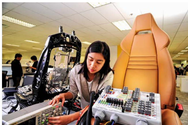
Victoria PENAS Senior System Test Engineer carries out system testing for seat heating and ventilation, as well as headrest and backrest adjustment
