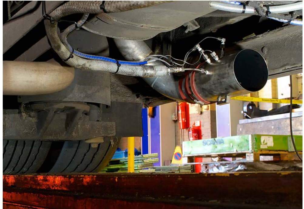
Instrumentation of the exhaust systems was entirely within the vehicle profile for testing on public roads
