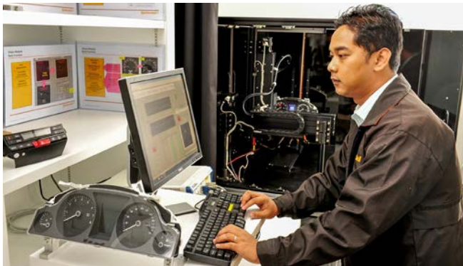
Tint Soe MIN Test Engineer Automated is managing a system designed to perform instrument cluster functional checks and measurements continues to be an ideal location for Continental to develop new products and systems for Asia and beyond. "
