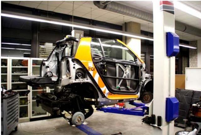
The University of Applied Sciences in Cologne retrofitted the compact car and installed plastic plain bearings from igus. (Source: igus GmbH).
