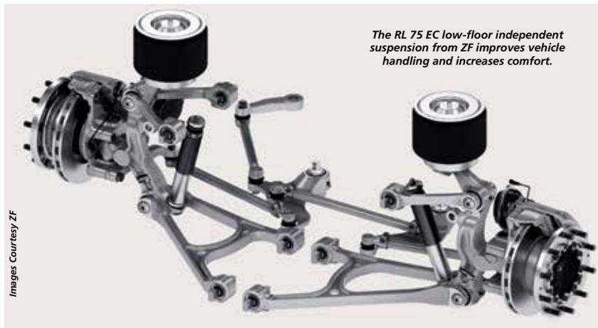
The RL 75 EC low-floor independent suspension from ZF improves vehicle handling and increases comfort.
