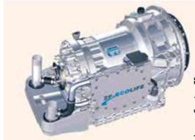
Since the ZF-EcoLife always keeps the engine in a low speed range and shifts up early, fuel consumption is reduced by up to ten percent. At bus stops, buses with this kind of transmission are perceived to be significantly quieter.
