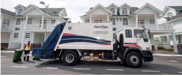
The robust driveline consists of a 280-hp six-cylinder in-line engine and a nine-speed overdrive gearbox. The vehicles are equipped with a wear-free exhaust valve brake, which enhances engine braking and lengthens the service life of the service brake.
